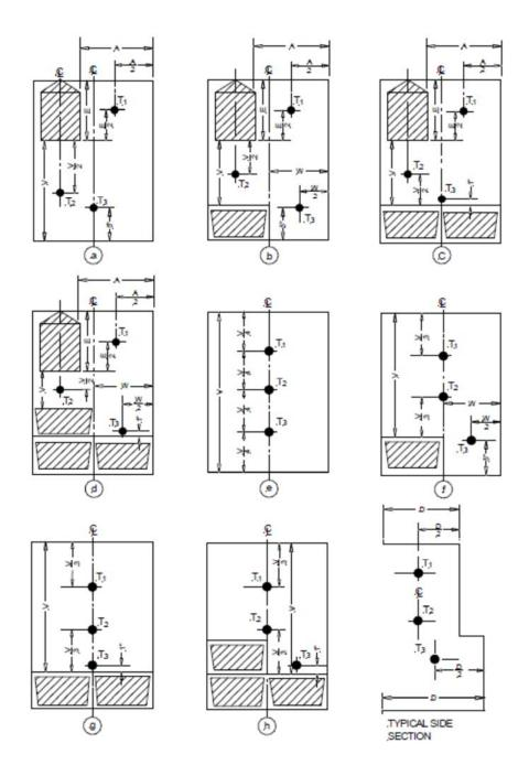
"A", "D", "E", "W" and "V" are arbitrary designations for determining location at which temperatures are to be measured. The depth dimension shall be measured from the back of the liner to a plane defining the gasket sealing surface. T1, T2 and T3 indicate thermocouple locations.
